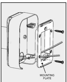
Attach the mounting plate to the antiknock shield with the 8 x 25 Pozi-drive screws supplied in the antiknock shield kit SOLOAKS0V1
