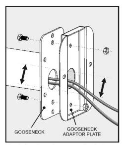
Feed wires through gooseneck adaptor plate. Ensure wire exits are aligned and fasten the adaptor plate to the gooseneck with Hex Screws and Nuts provided.
