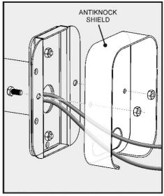
Feed the wiring through the antiknock shield and fasten it to the gooseneck adaptor plate assembly with the screws and nuts provided.
