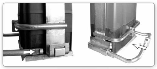
7. Fit the front bar to the assembly by feeding both legs of the bar through the bracket and overstrap.
