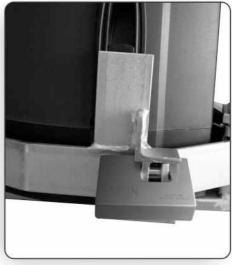
16. Finally, secure the cage by locking the left and right hand side straps together. A padlock with a 13mm diameter pin and 25mm 'throat' is recommended, (often referred to as a '78mm' lock).
