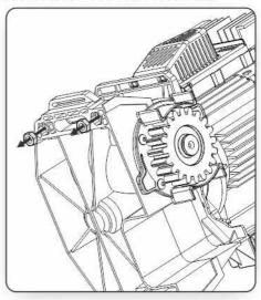
Remove all four captive nuts from the underside of the gearbox as shown. These are no longer required, as the threaded holes in the cage baseplate serve for height adjustment.
