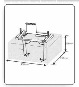
Ensure that the foundation plate has been properly installed. Refer to the Installation Manual for details.
