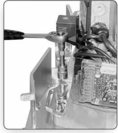
8. Assemble nut, spring washer, and load spreader onto the mounting bolts.
