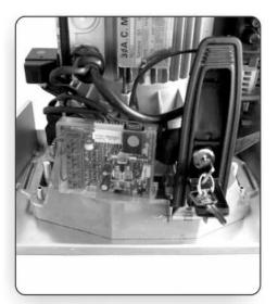
Place the gate motor over the base plate, making sure that the four grub screws and two mounting bolts from the foundation plate fit through the gate motor as shown.
