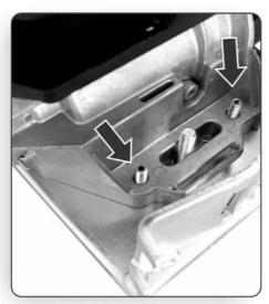
Adjust the height of the gate motor by tightening the four socket head grub screws equally; making sure the gate motor is level once complete.
