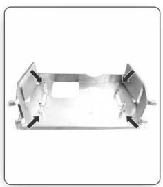
Screw the four M8x40 socket head grub screws supplied with A10/D10/D10 Turbo into the threaded holes in the base plate.
